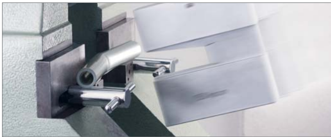
Fig. 3-2 Universal pipe RAUTTAN flex in the notch impact testing device
