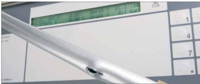
Fig. 3-1 Results of a burst pressure test with the universal pipe RAUTTAN flex
