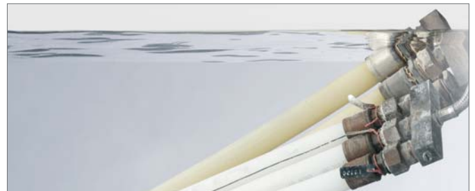
Fig. 3-4 Pipes in a long-term test (under pressure in a water bath)
