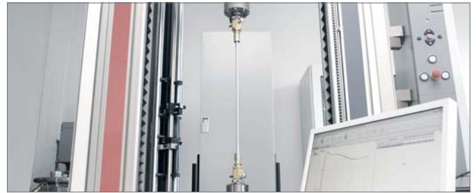
Fig. 3-3 Procedure of a tension test
