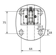
Dimensions of base-plate for Clamped Floor Bracket FK
