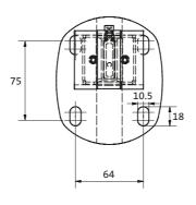
Dimensions of base-plate for Floor Bracket SK
